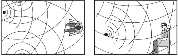
**Figure 9-10.** Even though they suffer from “venetian blind” effect, angled multiple panel speakers can deliver good imaging, but only to specific spots in the listening area.
