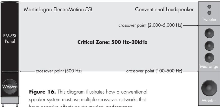
**Figure 16.** This diagram illustrates how a conventional speaker system must use multiple crossover networks that have negative effects on the musical performance.
