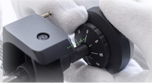
**16** Turn the counterweight counterclockwise until the scale reads roughly 18.
