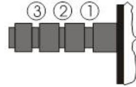
Screw ANTI-SKATING STUB into the pre-drilled hole here:
