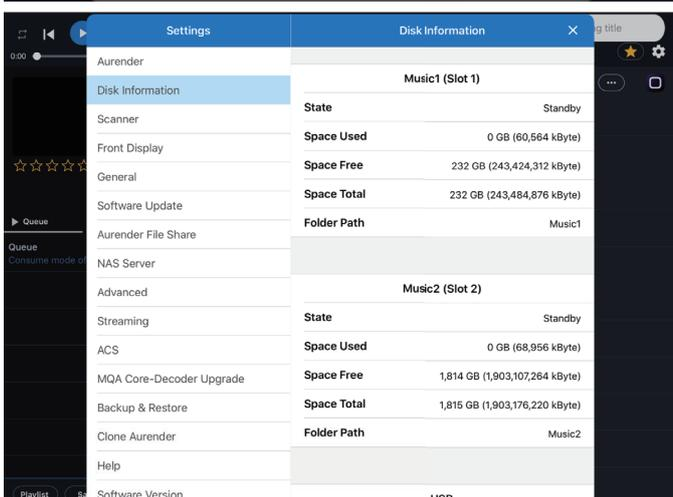
8. After formatting is complete and the Aurender has rebooted, confirm that the newly installed and formatted drive[s] are recognized by checking "Disk Information" menu.
