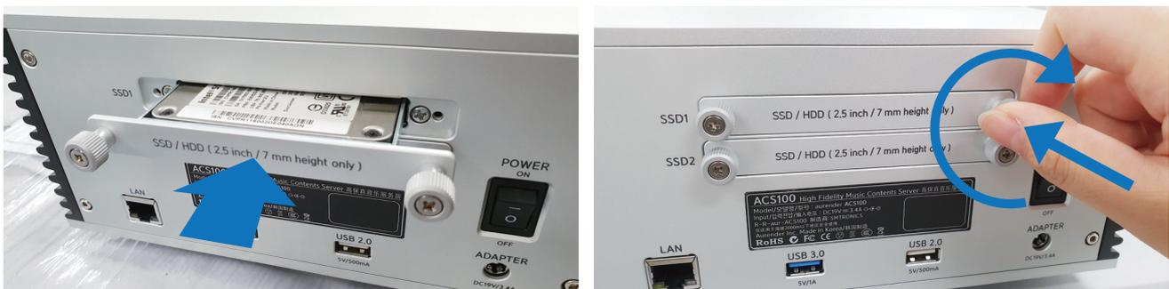
3. Gently push the tray[s] containing SSD[s]/HDD[s] into the slot.
