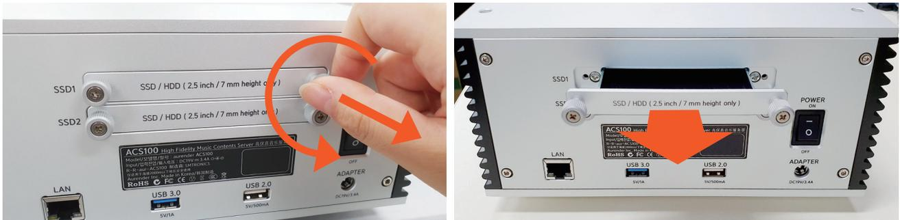
1. Unscrew and eject the disc enclosure tray[s] before turning the unit on.
