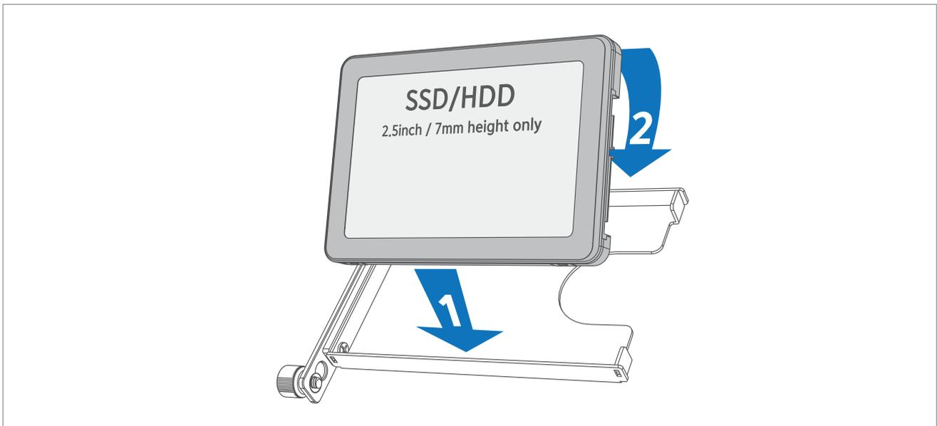
2. Install SSD[s]/HDD[s] into the tray[s] as pictured.
