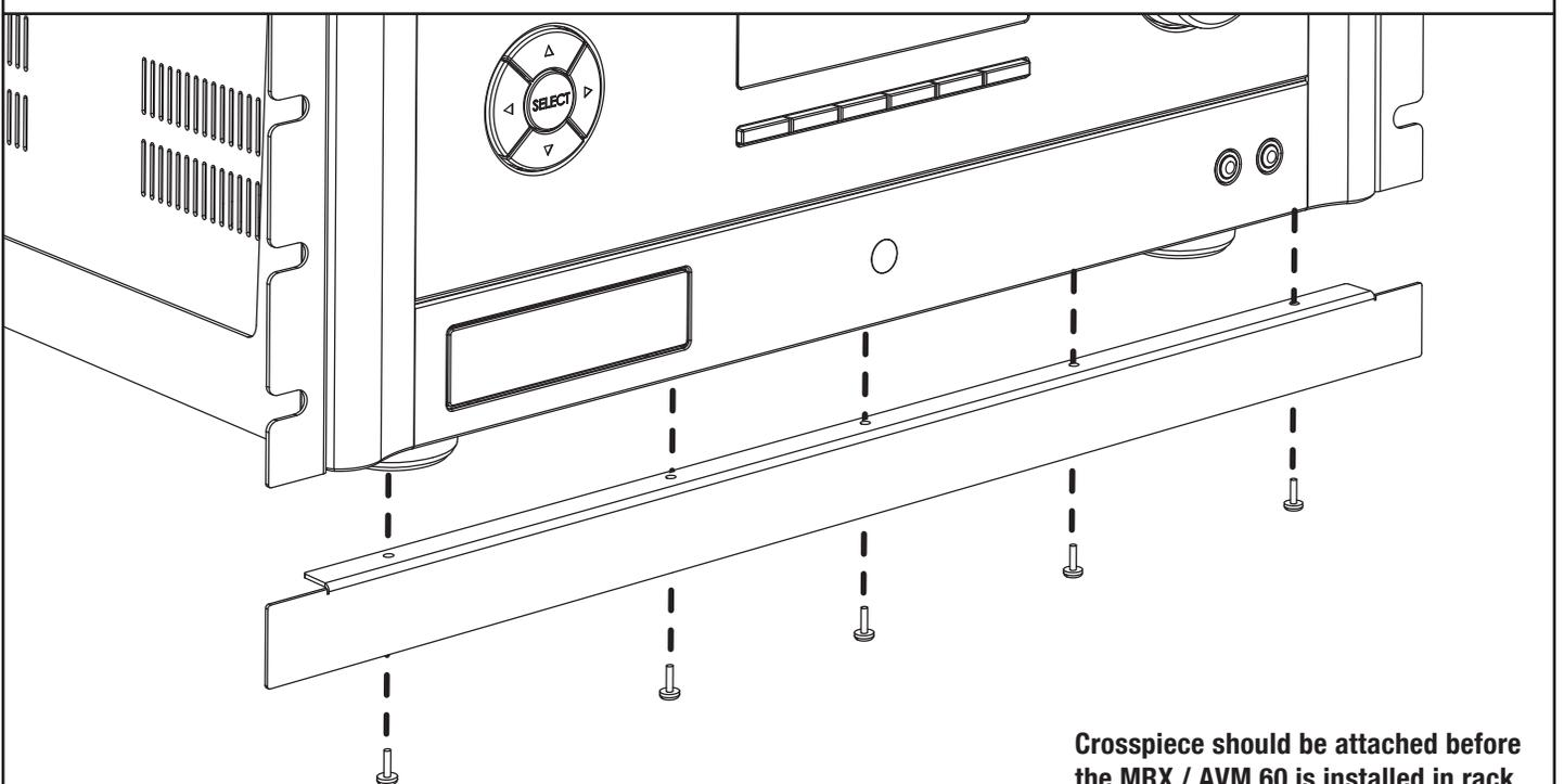
Crosspiece should be attached before the MRX / AVM 60 is installed in rack.
