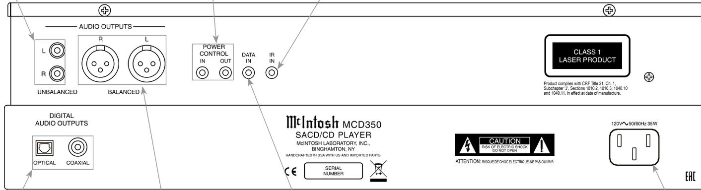
DIGITAL AUDIO OUTPUTS OPTICAL and COAXIAL send a Digital Audio Signal to a Preamplifier or an A/V Control Center with a D/A Converter or a decoder
