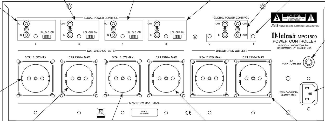
SWITCHED AC Outlet controlled by LOCAL POWER CONTROL number 6 Switch Setting and/or the received Power Control Signal
