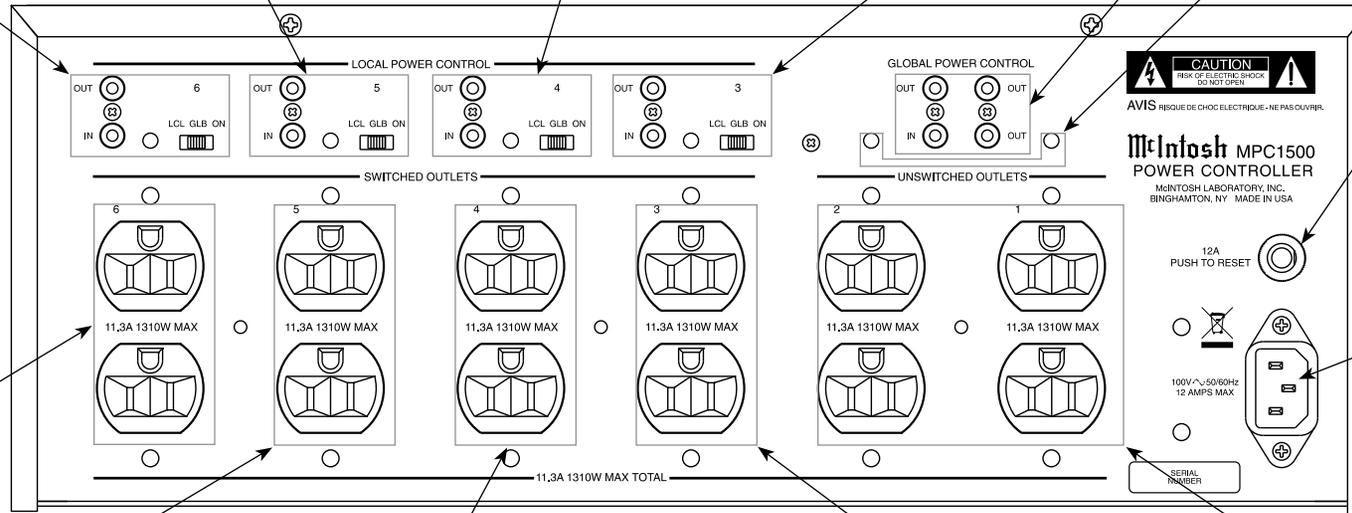
SWITCHED AC Outlet controlled by LOCAL POWER CONTROL number 6 Switch Setting and/or the received Power Control Signal
