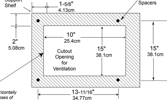
Note: Center the cutout horizontally on the unit. For purposes of clarity, the above illustration is not drawn to scale.
