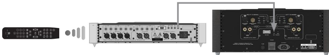
In figure 4 we have a 740P Preamp and 860A v2 amplifier connected together via their respective 12V triggers; The 12V trigger output on the 740P is connected to the 12V trigger input on the 860A v2 (using a 1/8" mini-jack cable). When you turn on the 740P via remote control (or its Standby button), the 860A v2 will turn on automatically. The same rule applies when you put the 740P into Standby mode.
