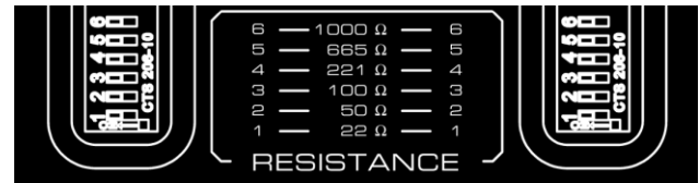
Figure 3: Left and right channel DIP switches for resistance loading adjustments
