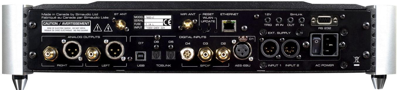
Figure 2: 780D v2 Rear panel
