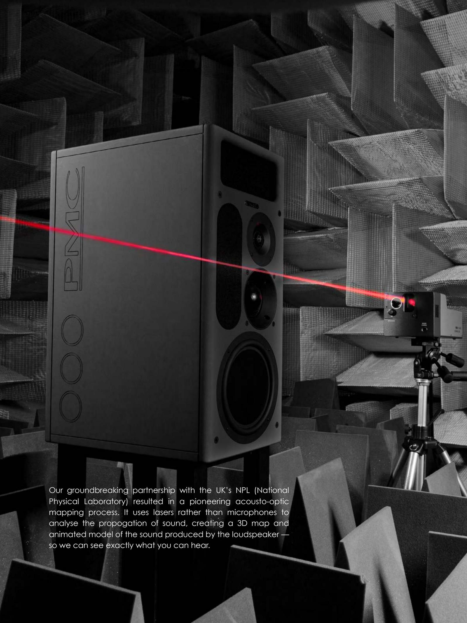
Our groundbreaking partnership with the UK's NPL (National Physical Laboratory) resulted in a pioneering acousto-optic mapping process. It uses lasers rather than microphones to analyse the propagation of sound, creating a 3D map and animated model of the sound produced by the loudspeaker — so we can see exactly what you can hear.
