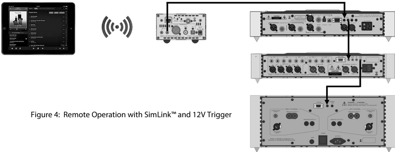
Figure 4: Remote Operation with SimLink™ and 12V Trigger
