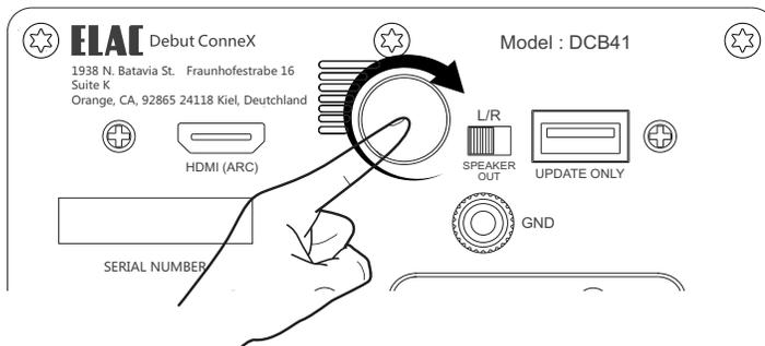
The Volume knob can be used to adjust volume, change input and power on.
