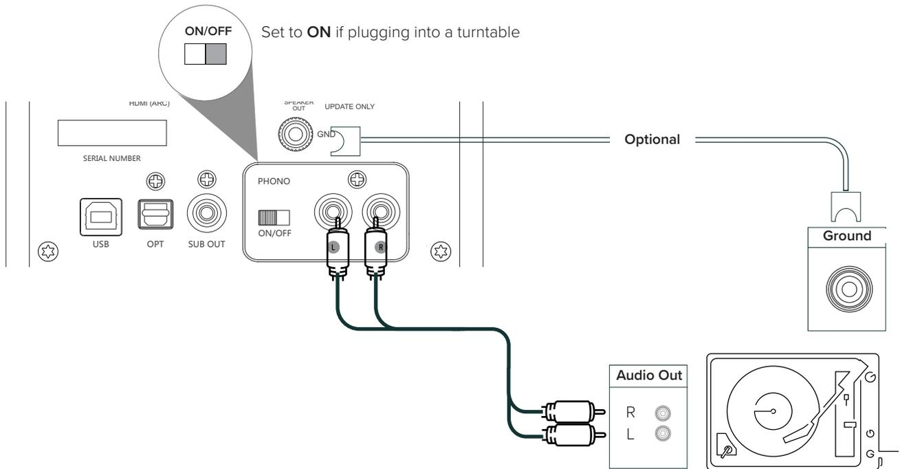
Note: Some turntables have built in phono pre-amplifiers that can be disabled. Ensure the turntable pre-amplifier is set to OFF and DCB41 is set to ON.
