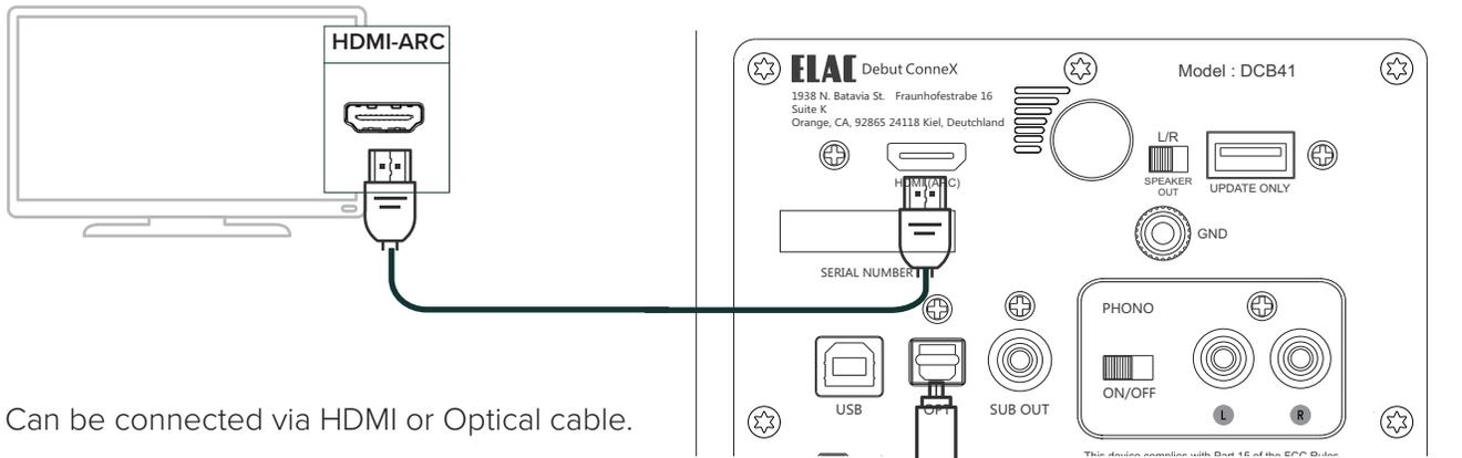
Can be connected via HDMI or Optical cable.
