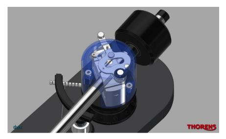
When changing a pickup, the arm only needs to be adjusted to the 0 point. The adjustment of the tracking force is generated by a spring which is located below the encapsulation of the tonearm. The azimuth angle is also set below the cover with a 2.5 mm Allen key. The internal highly flexible copper OFC wires were selected after careful hearing tests.
