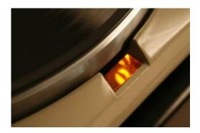
View of the plate stroboscope. The glow lamp casts its light in alternating current cycles
