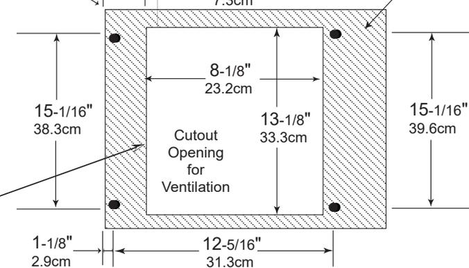
*Note: Center the cutout Horizontally on the unit. For purposes of clarity, the above illustration is not drawn to scale.*
