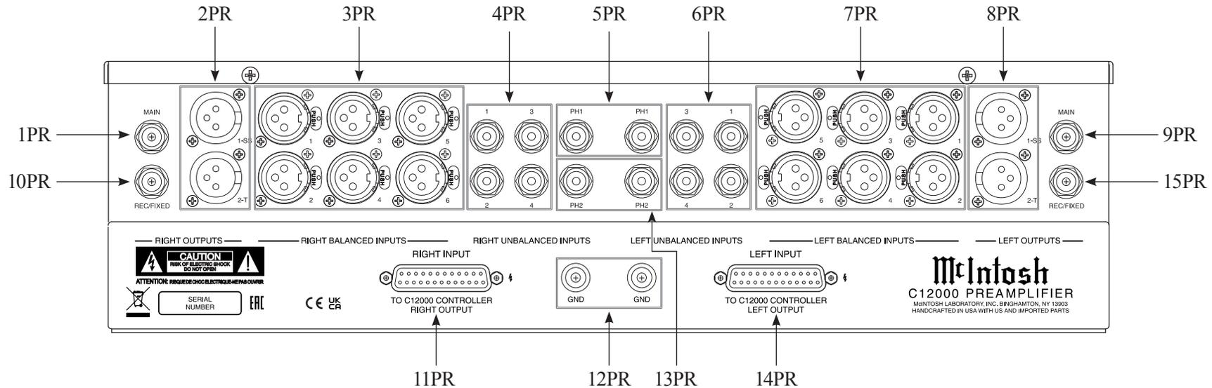
1PR RIGHT OUTPUT MAIN (Unbalanced) sends signals to a Power Amplifier - Can be configured to use Solid State or Tube amplification (see Page 29)
