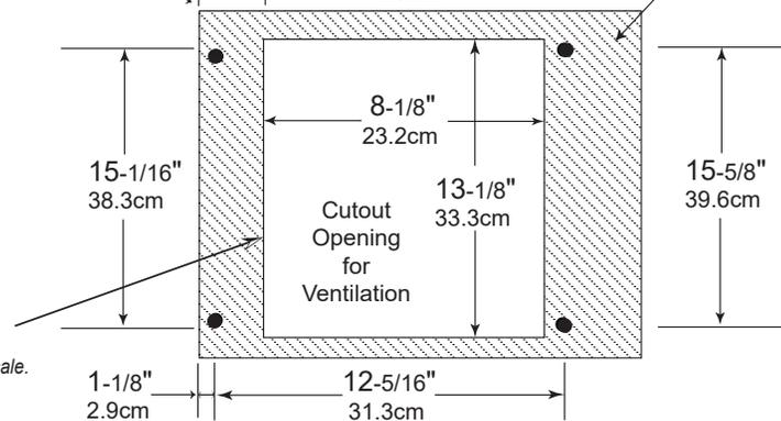
**Note:** Center the cutout Horizontally on the unit. For purposes of clarity, the above illustration is not drawn to scale.
