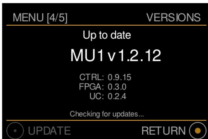
In this menu you can view the current software version and start an update. The MU1 automatically checks for an update every hour and also when entering this menu page from menu page [4/6]. If the MU1 is checking for updates, this is shown at the bottom of this menu.
