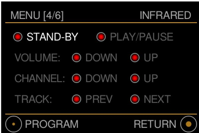
The dot will turn orange until the MU1 receives an infrared command. Press the desired button on your infrared remote to connect this infrared command to the selected function. When the MU1 receives an infrared command the dot will turn green and it returns to the infrared selection menu as shown in the previous image.
