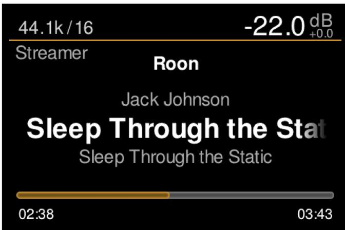
If an LS1 is connected, the MU1 will send volume control data to the DSP of the LS1 via its proprietary cat5 cable. If volume control is activated for one or more digital outputs, the FPGA chip performs a volume attenuation at high precision for these output(s). See 'Settings menu [3/6]' for selecting volume control on the digital outputs.
