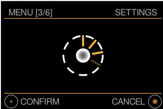
Turn the main knob clockwise to increase the brightness and anti-clockwise to decrease the brightness. Please note that the LED can not be turned off completely to facilitate showing whether the MU1 is in operation/stand-by or power off.
