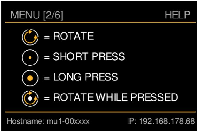
This Help menu shows the pictograms that are used in the MU1 for operating the main knob. At the bottom of the screen the current network information is shown. The indicated hostname depends on the serial number of your MU1. If the IP address shows 'unknown', there is no network connection and in that case the MU1 cannot be found by the Roon App in your tablet or smart phone. Please check the network connection of your MU1.
