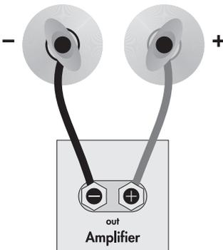
**Fig. 1b:** Single-wire connection.
