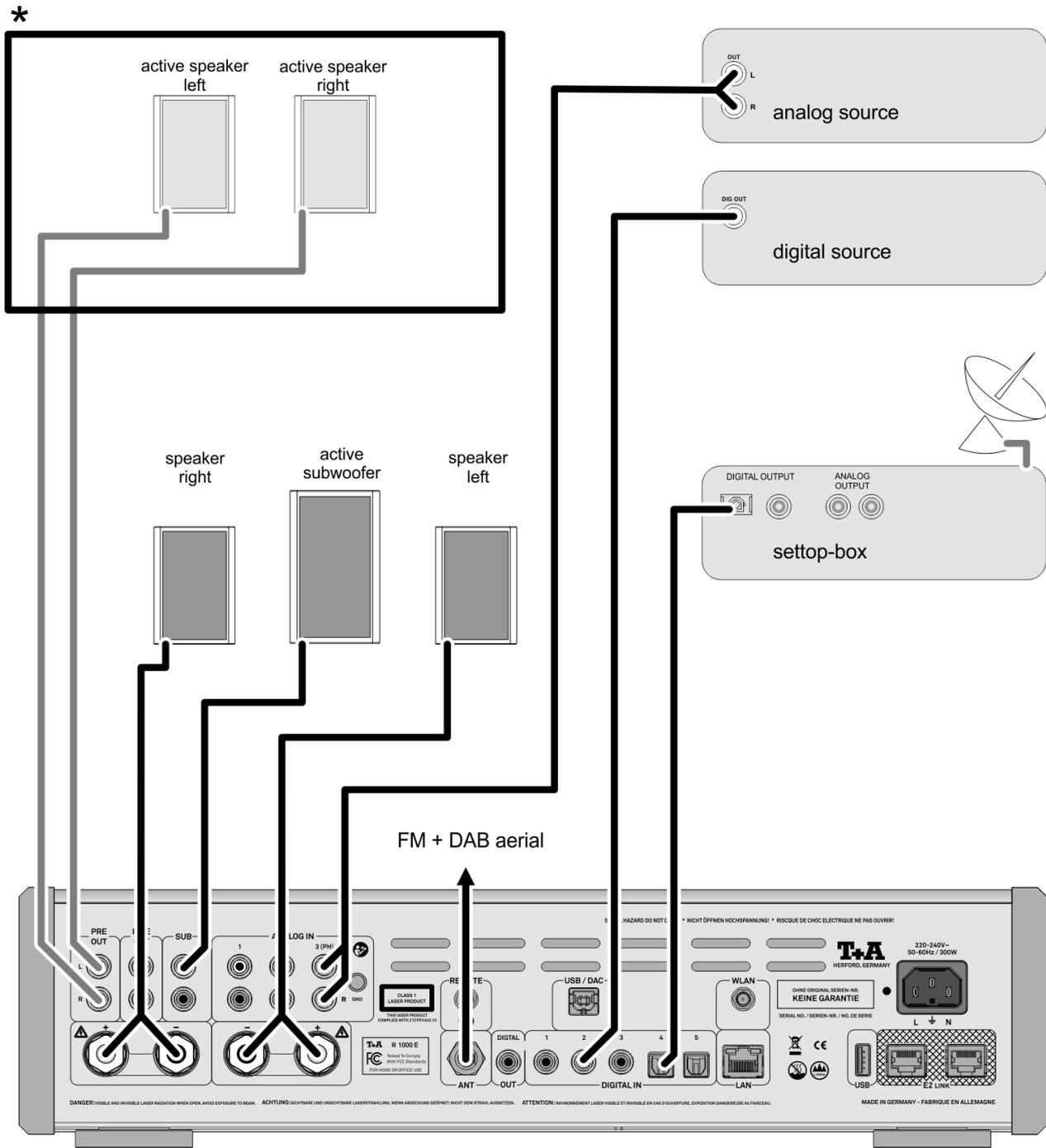
\* As an alternative to passive loudspeakers it is possible to use active speakers, which are connected to the pre-amplifier output.
