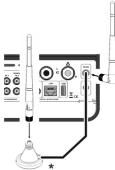
\* The aerial can also be set up free-standing using the magnetic base supplied in the set; this ensures maximum possible range.
