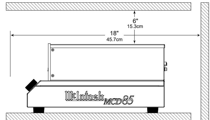
Figure 02– Ventilation requirements
