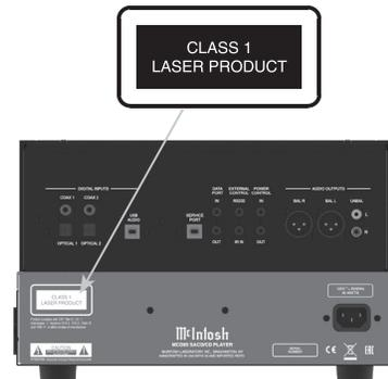
**CAUTION:** CLASS 3R INVISIBLE LASER RADIATION WHEN OPEN. DO NOT STARE INTO THE BEAM OR VIEW DIRECTLY WITH OPTICAL INSTRUMENTS. AVOID DIRECT EYE EXPOSURE.
